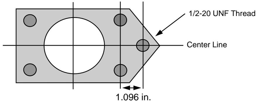
If you do not use high steer or do not want to modify 4 hole steering arms, simply do not use this bolt hole. A short 1/2" 20 bolt can be used to plug the unused hole and to keep it clean and free of debris.
